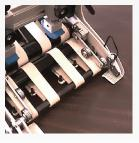
Our Patented paper guide extensions guide the document right into the gripper, eliminating extra components and touchy photo eye adjustments!
